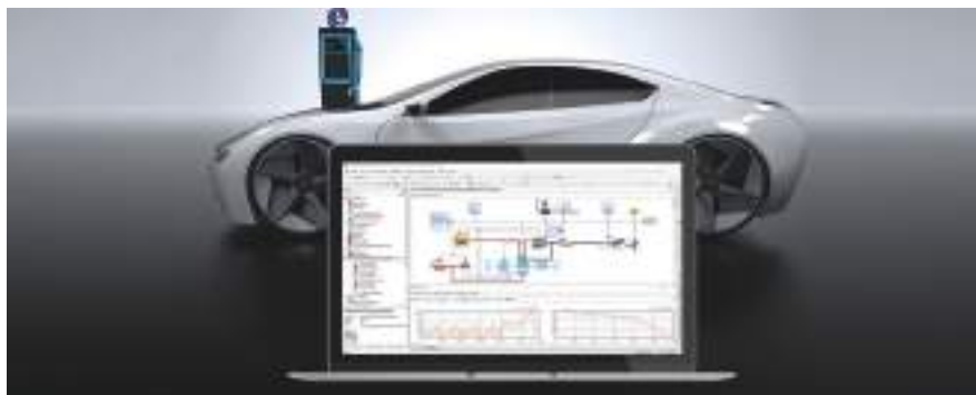
ESI's SimulationX model of an electric vehicle including Worldwide Harmonized Light Vehicle Test Procedure (WLTP) driving cycle, cooling system for the battery and the electric machine, as well as the cabin heating and a driver model
