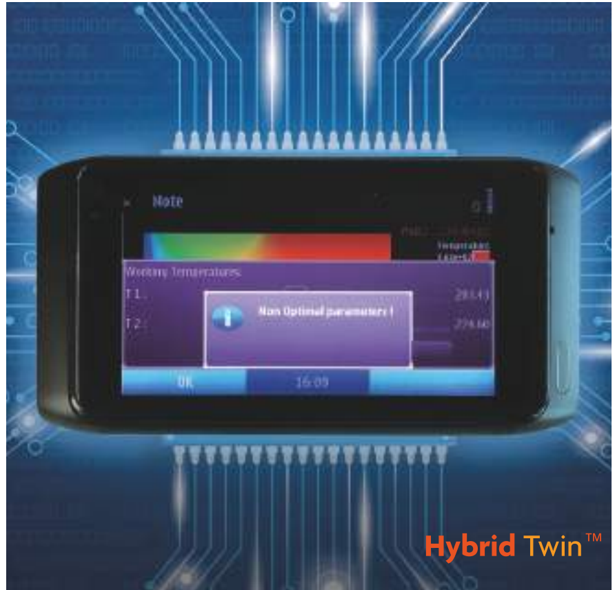
Reduced thermal model on a hand-held device. From the collected data, the model detects that the system is ill-functioning, as the real parameters are different from the nominal (optimal) ones.
