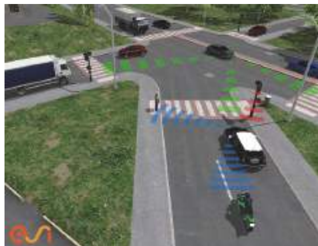
ESI Pro-SiVIC™ allows OEMs to virtually test the operational performance of various perception systems (sensors) onboard a vehicle, thereby supporting the development of functions such as Advanced Driver Assistance Systems (ADAS) and Autonomous Driving
