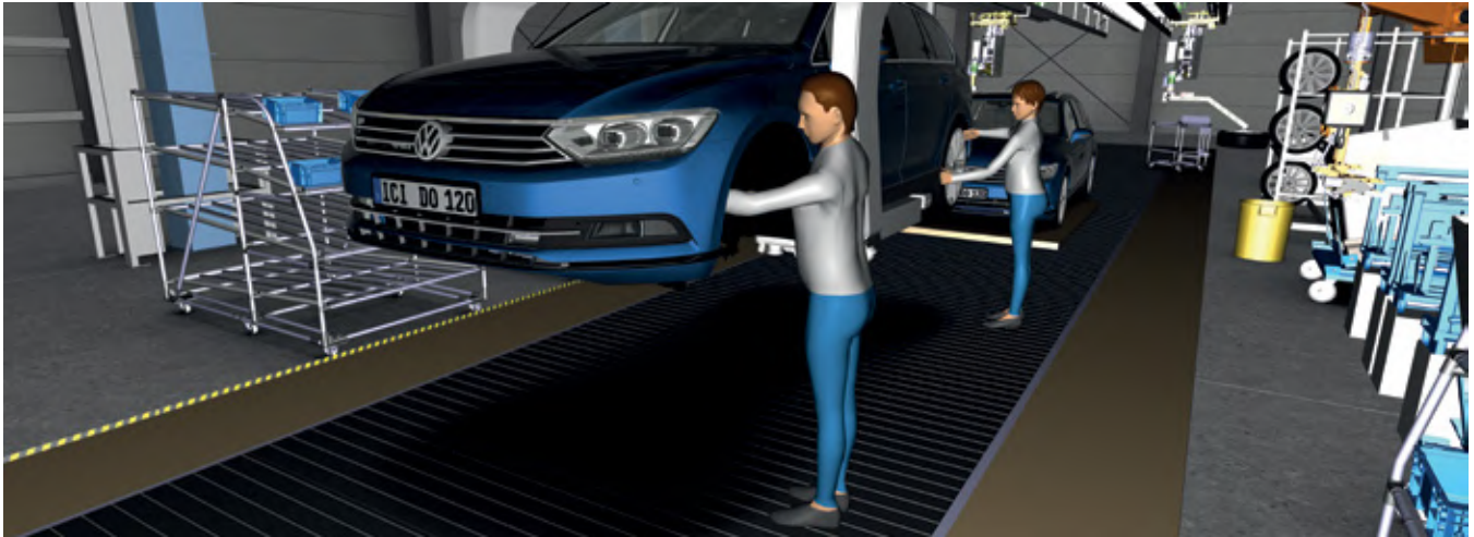
Experience assembly & capture process with Digital Human Model(s). Model data is Courtesy of Volkswagen
